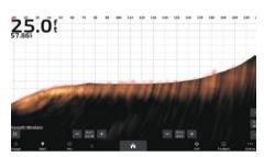
To help give you time to avoid collisions with submerged obstacles, FrontVü shows underwater obstructions within a 300-foot range as you approach them in real time<sup>2</sup>.
