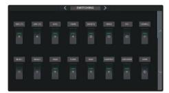
Get control and protection of up to 20 circuits via your chartplotter rather than a physical button or switch.
