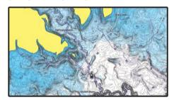
Shallow water shading for a user-defined depth gives a clearer picture of shallow waters to avoid when navigating.
