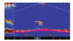
Shows real-time moving sonar images of small baitfish and large target fish swimming below your boat and pinpoints their distance left or right and their depths.
