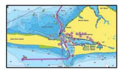
Built-in Auto Guidance+ technology¹ uses your desired depth and overhead clearance, along with chart data and frequently traveled routes, to calculate a suggested path to follow from dock to dock. This results in smoother, more detailed routes, and it now calculates even faster.
