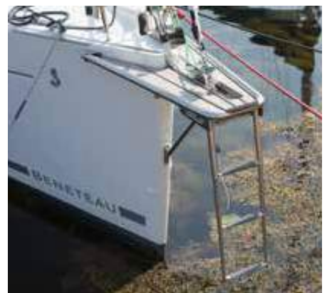
The PB120 bowsprit allows for the combination of a 20 kg anchor with the BKT73A telescopic ladder in casing.
