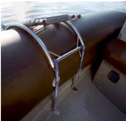
The RIB ladder is resting on the boat's tube and is secured with two straps.
