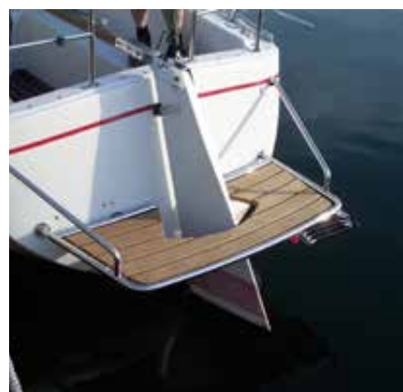
PR1306030 for sailboats with surface-mounted rudder.
