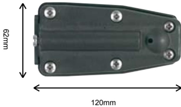
**Luff boxes.** Series 35 luff boxes connect to the slide with a cleverly concealed M10 nut that provides a solid connection and full lay flat rotation of the batten. The long housing ensures the batten remains in place while the supplied batten guides allow the choice of either 10mm round or 30mm flat battens and provide the additional benefit of an integral screw tension adjusting system.
