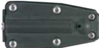
**Series 55 luff boxes** connect to the slide's hinged arm using an M10 thread. Battens can be easily removed from the luff end by removal of the cover plate. They are moulded from tough high grade Nylon and are supplied with three covers to allow the choice of 40mm flat, 30mm flat or 12m round batten.
